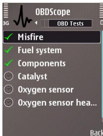
Figura 3: Tests OBD.
